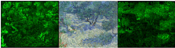
Fig. 19. Element map for copper (left) and chromium (right). Differences in how Van Gogh employed emerald green (copper map) and viridian (chromium map) are evident by comparison with the green paint strokes in the painting.
